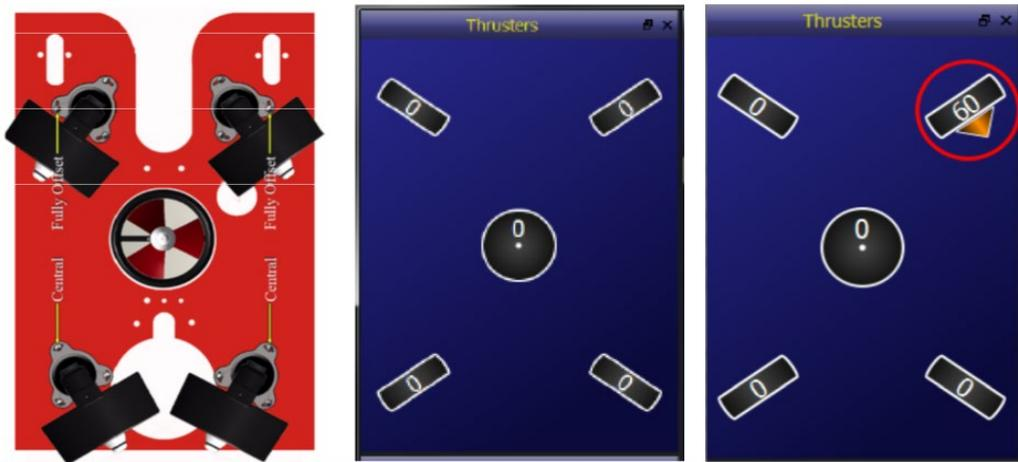
Figure 74: Schematic top view of ROV thrusters (left), Thrusters mounting position and angle with all thrusters idle (middle), and Thruster at 60% in a clockwise direction (right).
