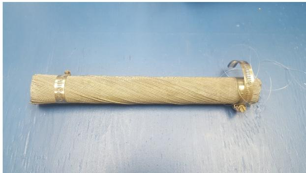
Figure 14: Armored umbilical cord (1.49 inch diameter).
