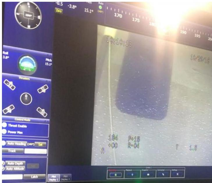
Figure 72: SAAB SeaEye Falcon 12423 touchscreen monitor displaying the video information from the camera and system information as widgets.
