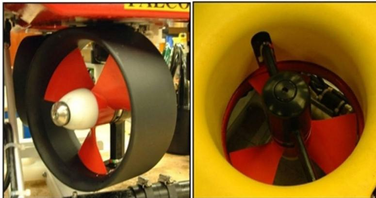
Figure 73: Horizontal (left), and vertical (right) thrusters.
