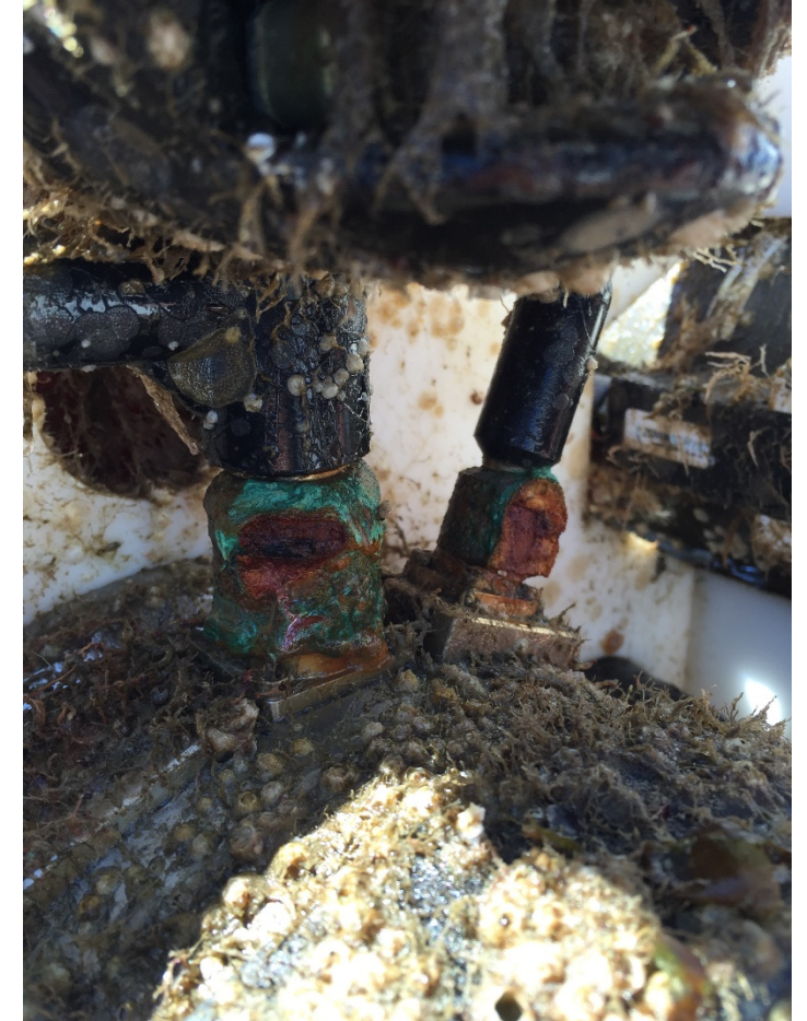
Examples of corrosion on anodized aluminum housing and connectors with dissimilar metals
